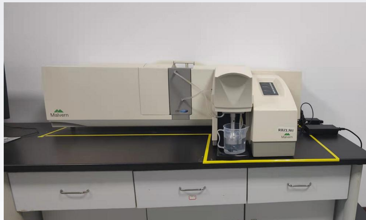
Malvern激光粒度检测仪 (原材料及浆料粒度检测) Malvern laser particle Detector
